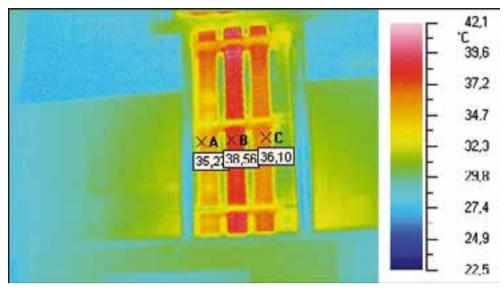
Figure (7). The middle bar is wormer of  $3^{\circ}C$  for higher load compared external bar.
