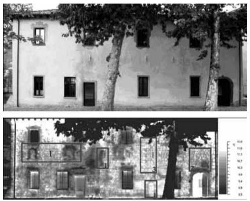
Figures 7 and 8. The Palazzo Marchesale in Melpignano (Lecce). The IR Thermogram magnifies the length and size of the smallest cracks (in the white squares).
